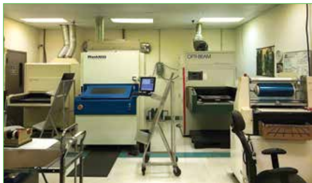
FIGURE 1. The yellow room at Prototron Circuits features a Maskless Lithography direct imager and Opti-Beam dry-film exposer.
