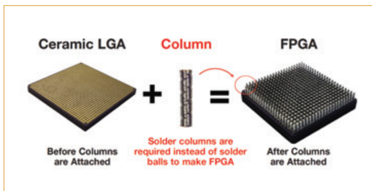
FIGURE 1. Sequence of FPGA package assembly with solder columns.
