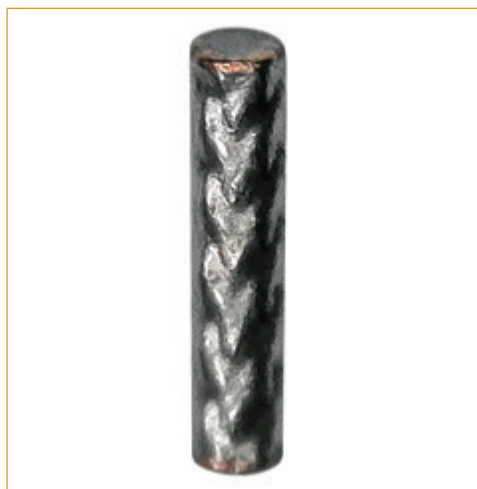
FIGURE 3. Braided solder column developed and patented by Topline.
