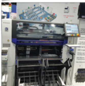
SPEED DEMON Yamaha's YRM20 dual-head placement machine.
