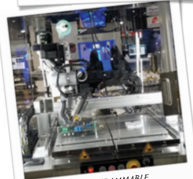
ALL PROGRAMMABLE Kurtz Ersa's Solder Smart five-axis soldering robot.
