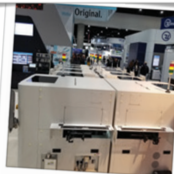
BACK TO BACK A pair of Hanwha printers feed a single HIM 520 placement machine.
