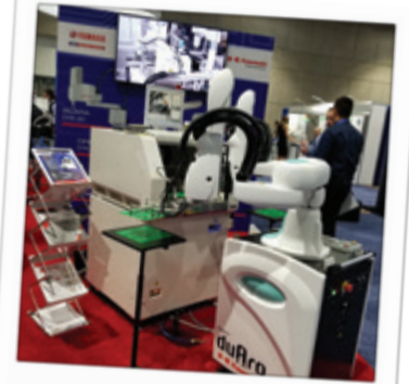
TWICE AS NICE The dual-arm Kawasaki Duaro RS robotic handler loads and unloads routers.
