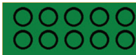
FIGURE 1. The clearance between pads and a surrounding copper plane is called a moat.
