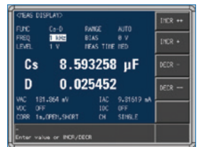
FIGURE 8. Capacitance measured without ALC. The testing level set to 1.0V; however, the voltage monitor shows only using 181.864mV.
