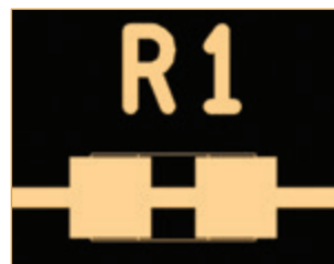
FIGURE 2. Series elements can be preplanned with common footprint geometry.
