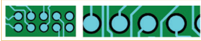
FIGURE 3. The autorouter might not center traces between pads or take an inefficient angle.
