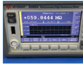
FIGURE 16. Insulation resistance measurement of a qualified MLCC using the B2987A electrometer/high resistance meter.
