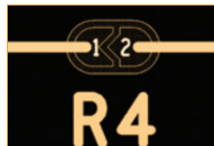
FIGURE 3. The additional border area enhances the jumper effect of this normally open circuit. Heating both sides permits a blob of solder to bridge the gap.
