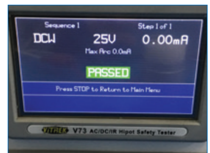
FIGURE 19. Dielectric withstanding voltage testing using the Vitrek V73 AC/DC/IR hipot tester showing the device passed the 2*voltage rating for the Class II MLCC part no. C2012JB1A476M125AC, which is expected for this class of MLCC.
