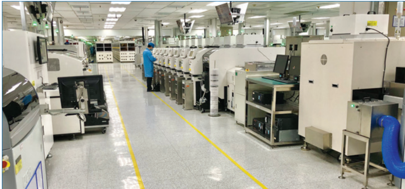
FIGURE 6. A single printer can feed eight SMT placement machines. USI says up to 400 highly dense SiP modules may be processed on a single substrate.
