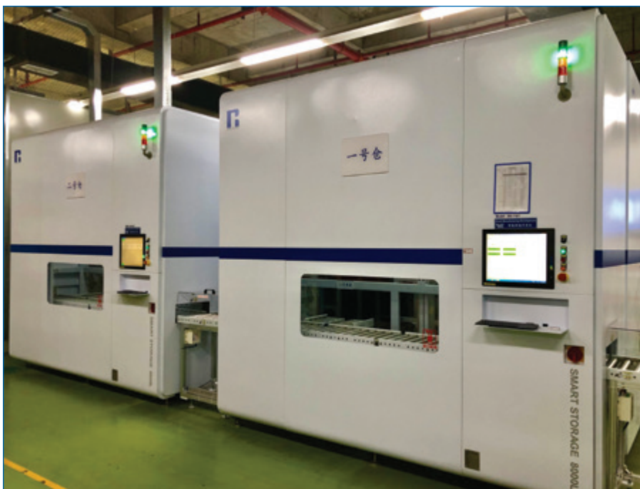
FIGURE 4. Parts are stored on reels inside intelligent storage systems in USI's component warehouses.
