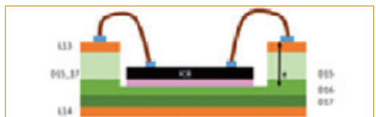
FIGURE 3. Custom ICs like wirebonds can be defined separately from the main board.
